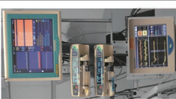
Figure 1. iControl-RP system with touchscreen user interface (top) showing various anesthesia parameters and waveforms. The system is connected to a patient's intravenous line and a Q-Core Sapphire Multi-Therapy Infusion Pump (Q-Core) (bottom) and NeuroSENSE (Sensory and Position) monitor.
